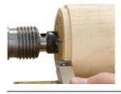
**Step 5** - Mount the tenon in a chuck. Support the opposite end with a revolving center.
